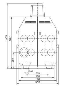
Dimensions by gravity outlet (Construction WS 8 G\* pictured)
